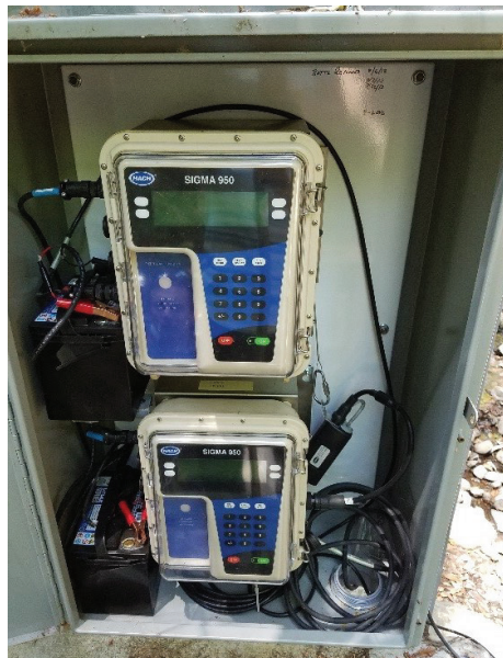
Photo of Asbury Creek diversion (left) and flow monitoring equipment (right: Asbury data recorders). Note the small pipe opening in the weir wall designed to allow 0.9 cfs stream flow to bypass diversion.
